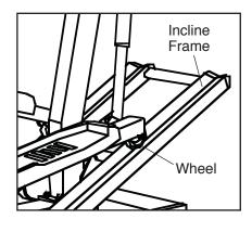
frame where the wheels make contact with it. Other parts of the elliptical crosstrainer can also be cleaned in this manner. **Never use abrasives or solvents.**
